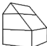
S3 - Woning 3-laags mank dak
