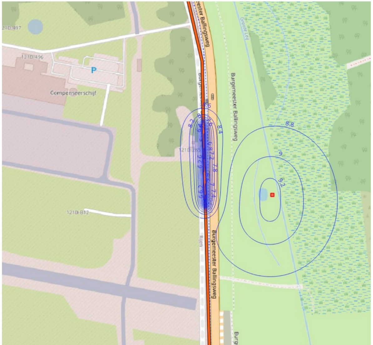
Figuur 4.2 Grondwatercontouren in [m NAP] Horizontale bemaling
