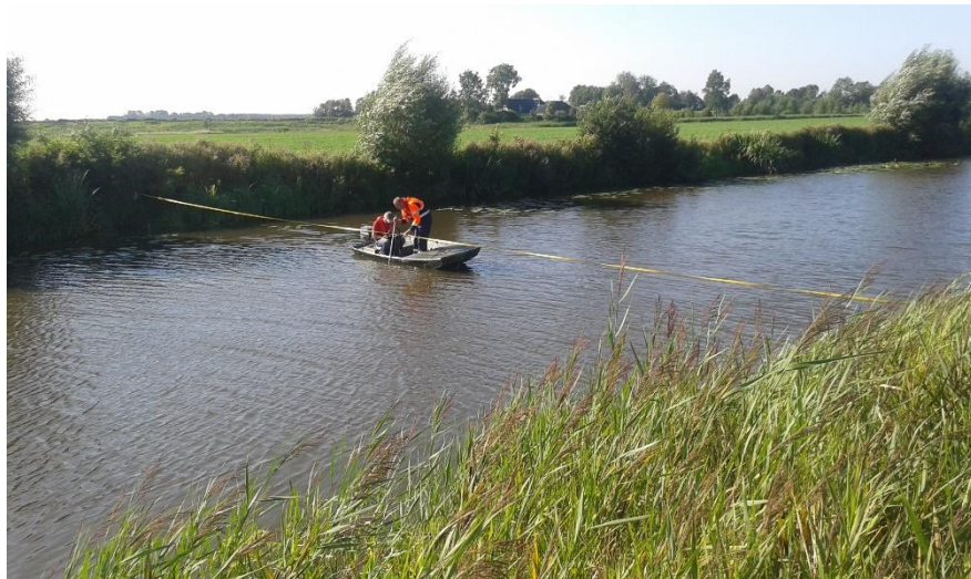
Handmatig inmeten watergang (foto: Antea Group)
