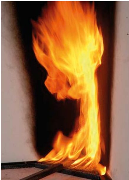
SBI fire test equipment in accordance with EN 13823
