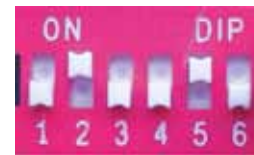
Block with 6 dipswitches
