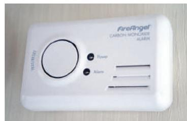
Check that the Carbon Monoxide (CO<sup>2</sup>) alarm is in working order. The green power light should flash every 50 seconds.
