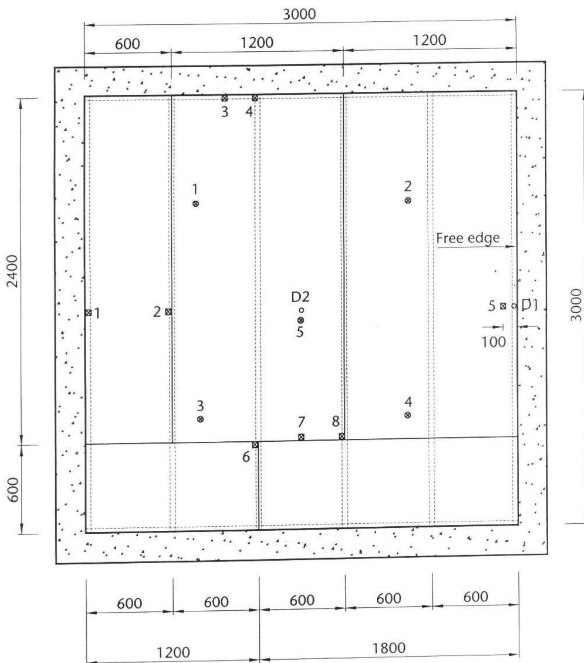
— Joints in the gypsum board layer
