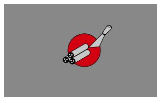
**Smooth CFS-IS.** Smooth before the skin forms using water and a spatula. Leave completed seal undisturbed for 48 hours.
