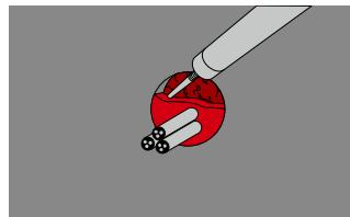
**Apply CFS-IS.** Apply to the required depth in order to obtain the desired fire rating. Making sure CFS-IS contacts all surfaces to provide maximum adhesion.
