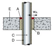
• Floor (E): Concrete or aerated concrete, minimum density of 550 kg/m³, minimum thickness 150 mm.
