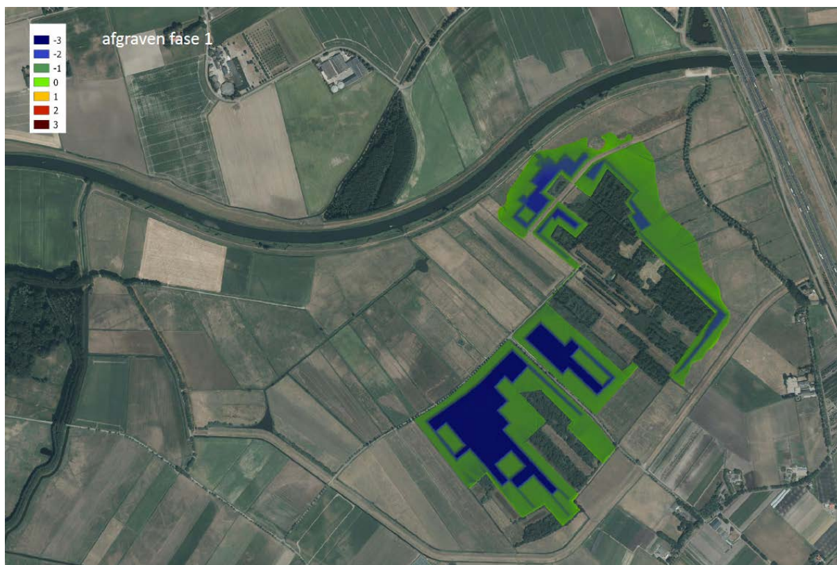
Figuur 2.12: Afgraving grond in meters Weimeren fase 1
