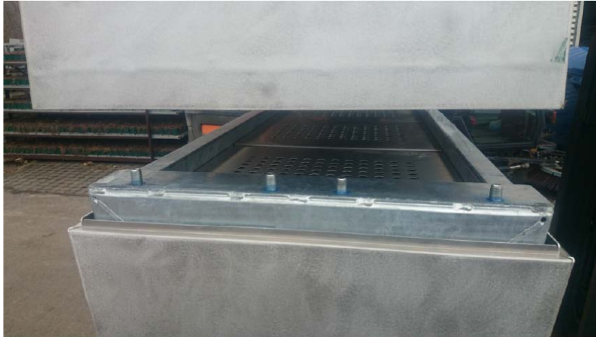
Figure 16: Connecting top with base
