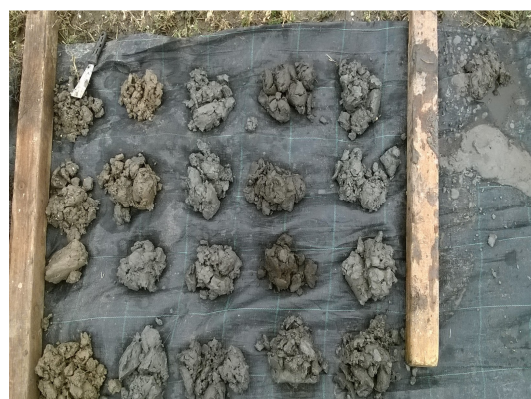
6. Boorlagen boring B-01
