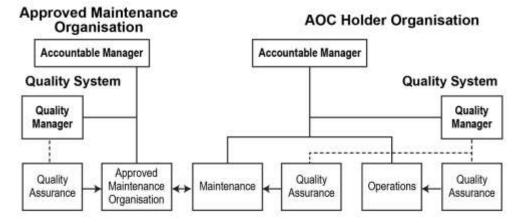
Note: The Quality System and Quality Audit Program of the AOC holder should assure that the maintenance carried out by the approved organization is in accordance with requirements specified by the AOC holder.
