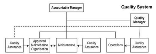
(b) Quality Systems related to an AOC holder's organization where aircraft maintenance is contracted out to an approved organization which is not integrated with the AOC holder.
