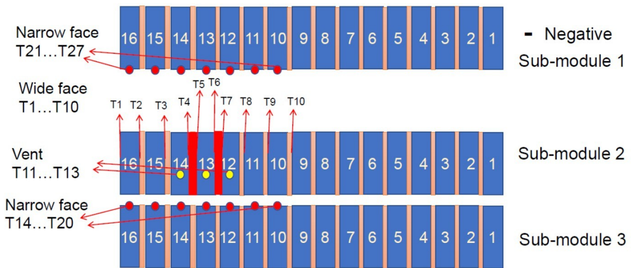
Figure 7. Thermocouple's locations outside module
