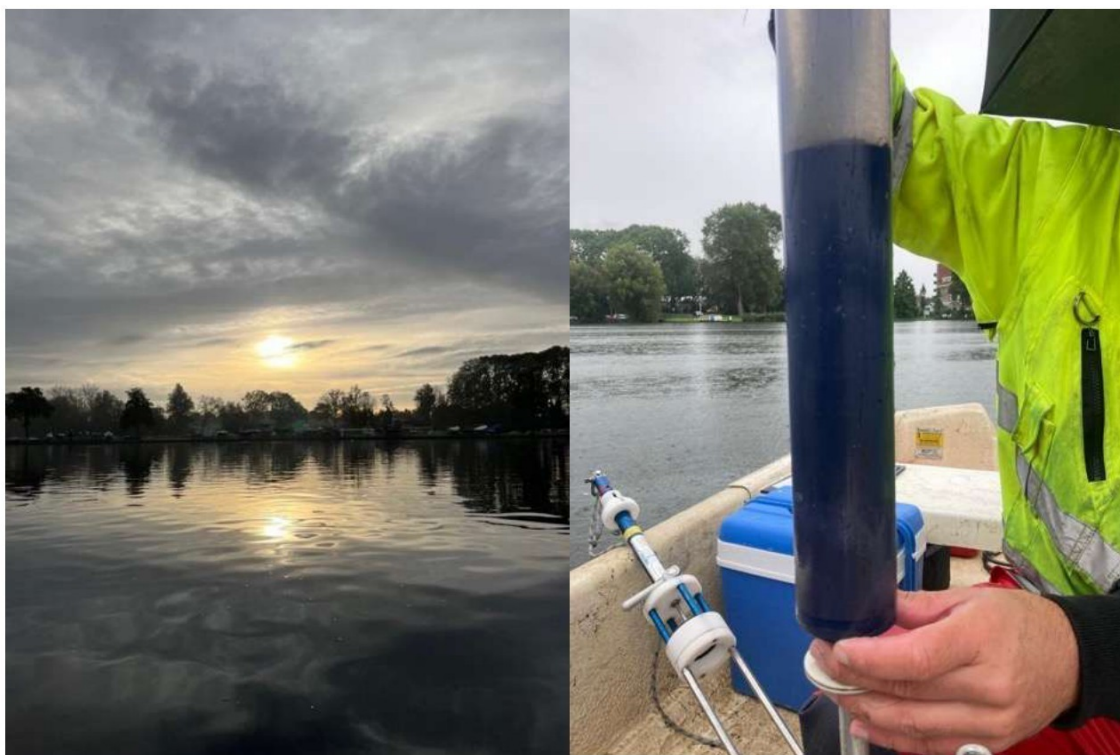
Figure 1: Sediment core sampling at Bergse Voorplas in Rotterdam using an UWITEC corer.
