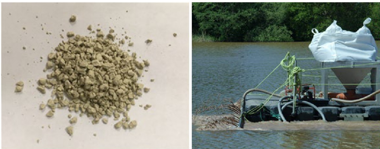
Figure 1. On the left, a picture of Phoslock® as a dry material and on the right Phoslock® being mixed with lake water and applied on the surface of Lake de Kuil (the Netherlands).
