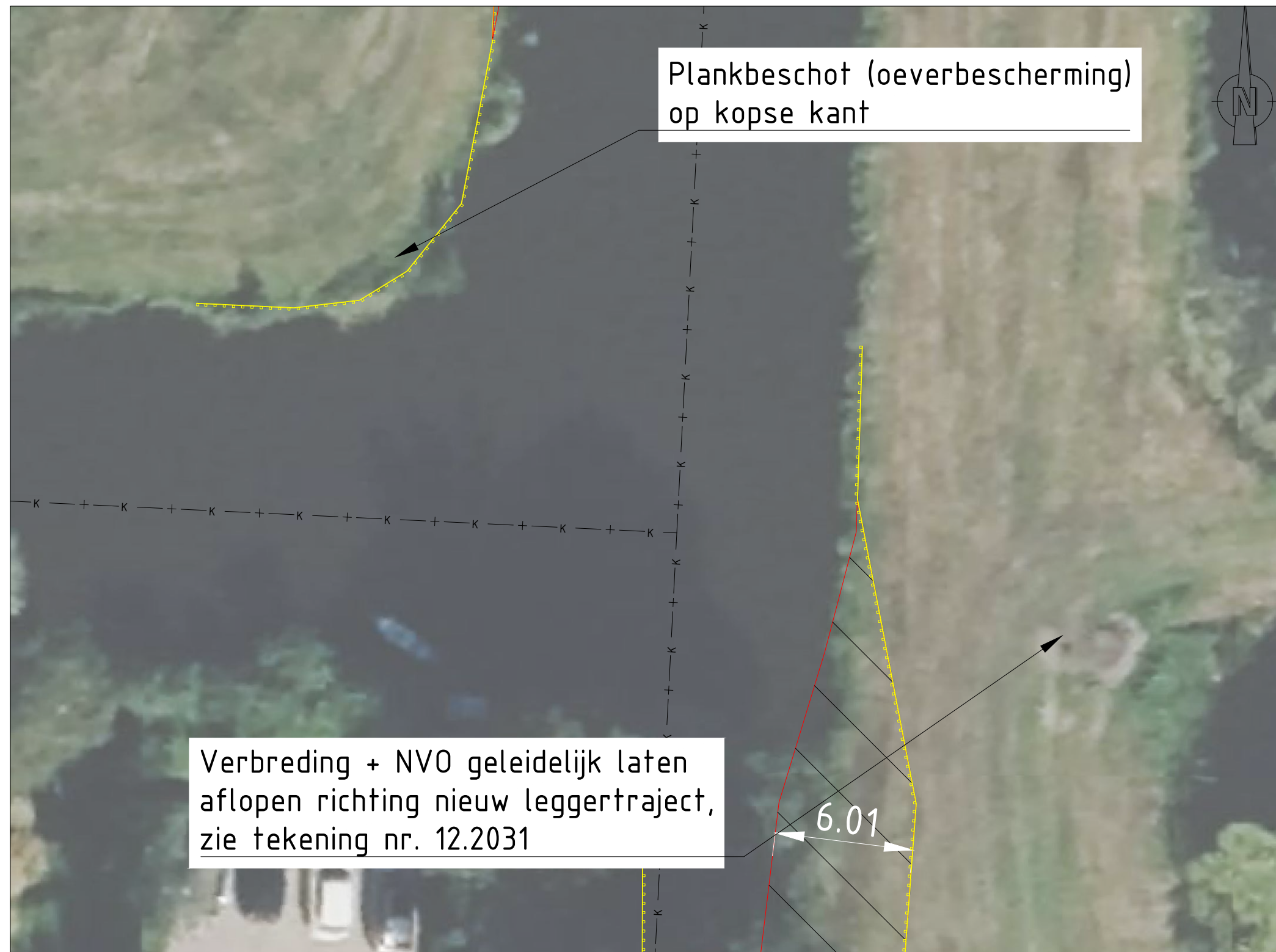
DETAIL B, LEGGERTRAJECT WOWA-58854+59830 SCHAAL 1 : 200
