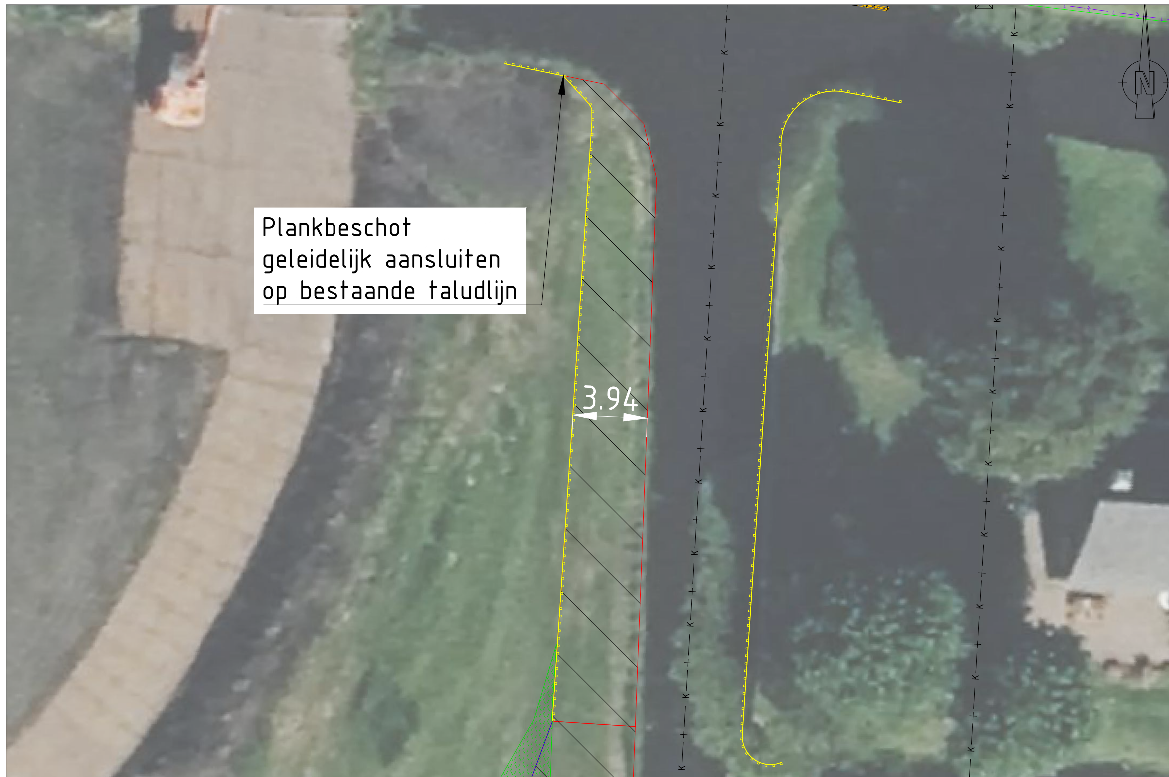
DETAIL A, LEGGERTRAJECT WOWA-58854+59830 SCHAAL 1 : 200
