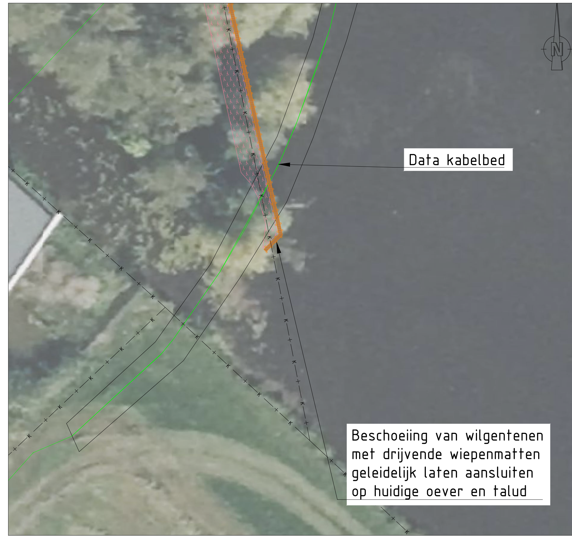
DETAIL A, LEGGERTRAJECT WOWA-69263 SCHAAL 1: 200
