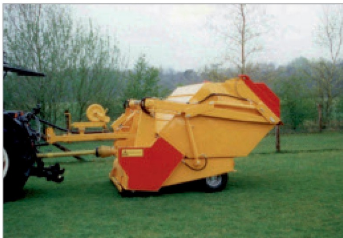
STH Phoenix PHK1800 veegmachine in hoogkippende uitvoering. STH Phoenix PHK1800 sweeper as high tipping model.
