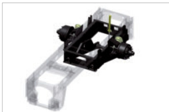
3 Dimensionale tekening van Ideal Chassis met Soil Protection onderstel. 3 dimensional drawing of the Ideal chassis with a Soil Protection carriage.
