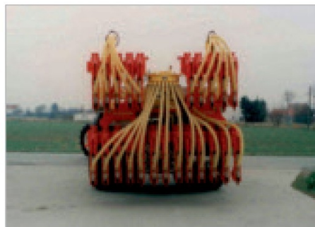
De Spider zodenbemester model SP560 met hydraulische transportopklapping. The Spider slurry injector model SP560 with hydraulic folding for transport.
