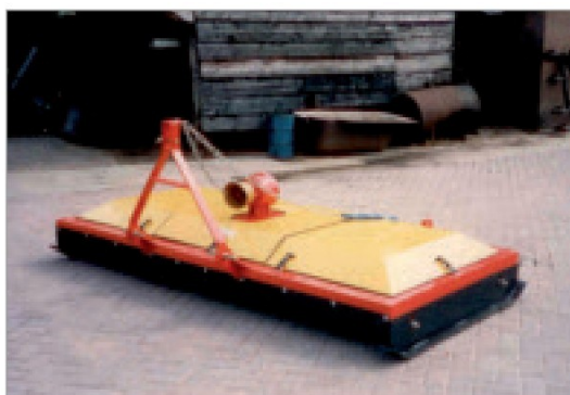
De UNI cirkelmaaier model UNI275, nog met stalen afschermkap zoals de eerste machines waren uitgevoerd. The UNI pasture topper model UNI275, still with steel shielding which was how the first machines were equipped.
