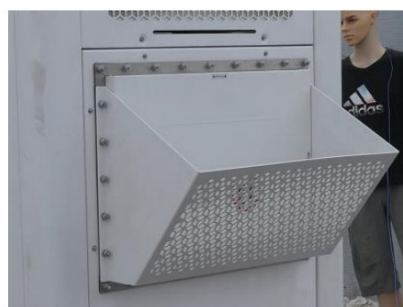
Figure8 Venting panel used in test
