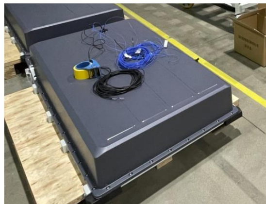
Figure12 Charged and encapsulated battery pack
