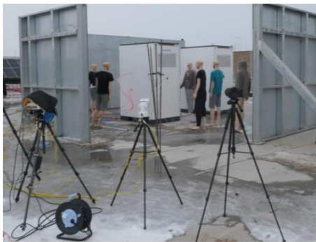
Figure19 Video data acquisition equipment
