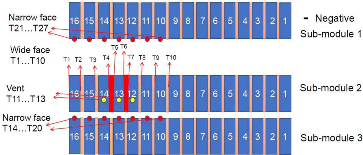
Figure 7. Thermocouple's locations outside module
