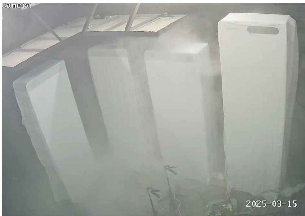
Smoke release from initiating unit
