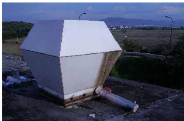
Fig. 4. Data sampling – tested bio-washer
