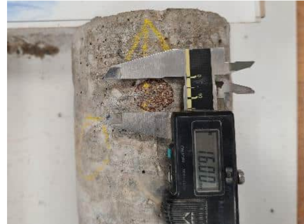
Foto 6.39: Diameter Ø 16 mm.
