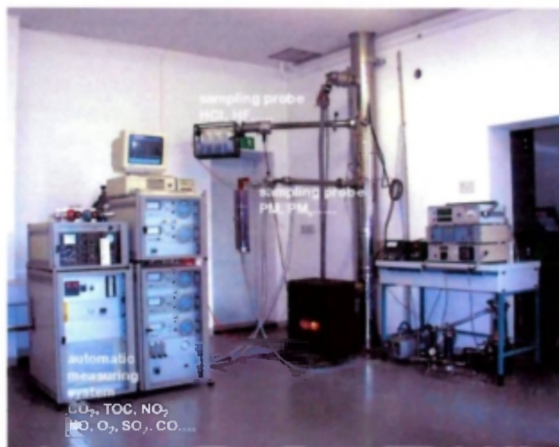
Fig. 1: Test arrangement household stove (brown coal briquette)
