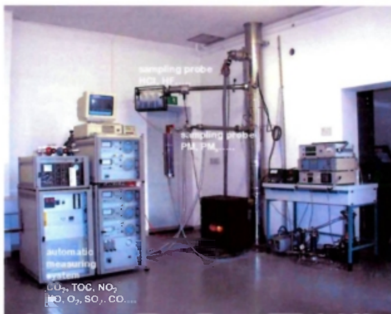
Fig. 1: Test arrangement household stove (brown coal briquette)
