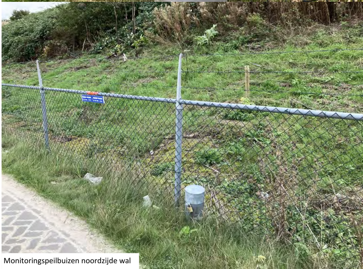
Monitoringspeilbuizen in RVS-koker
