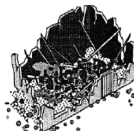
Damage Level: D5 Collapse Extent of Collapse: 100% of Volume
