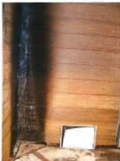
Photographs 3 and 4: Specimen with horizontal orientated planks after testing
