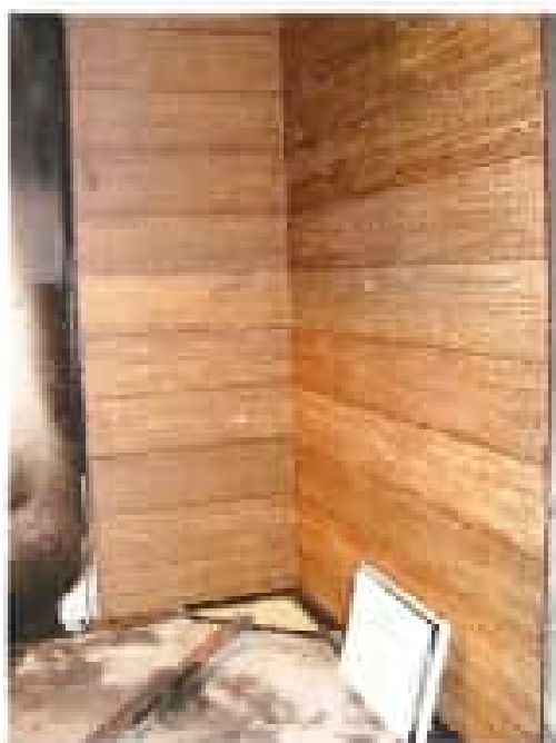
Photographs 1 and 2 : Specimen with horizontal orientated planks prior to testing
