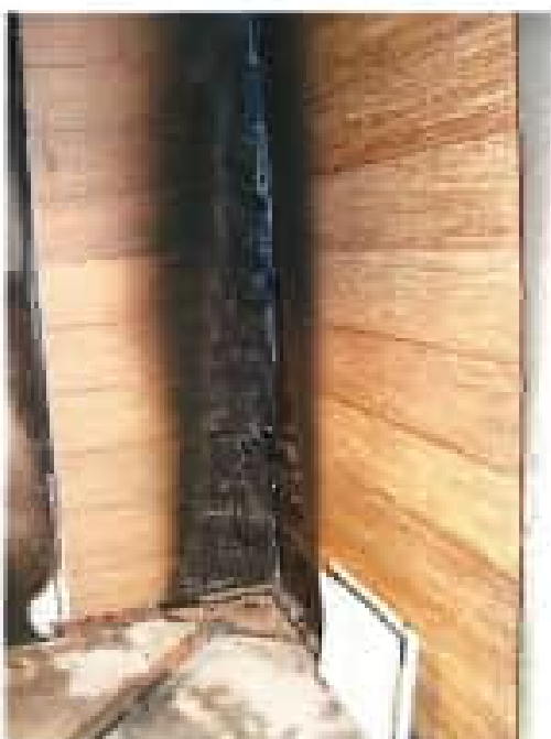
Photographs 3 and 4: Specimen with horizontal orientated planks after testing
