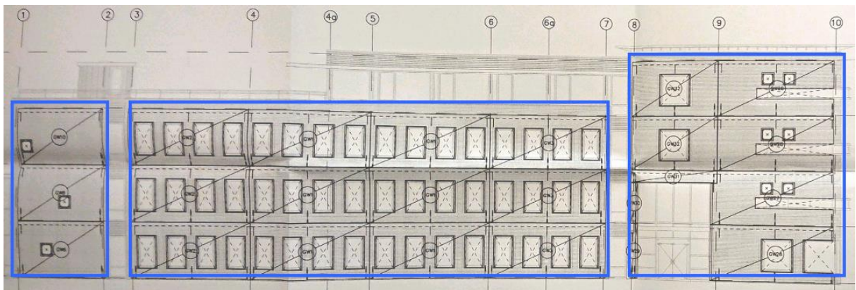
Prefab binnenbladen op as A
