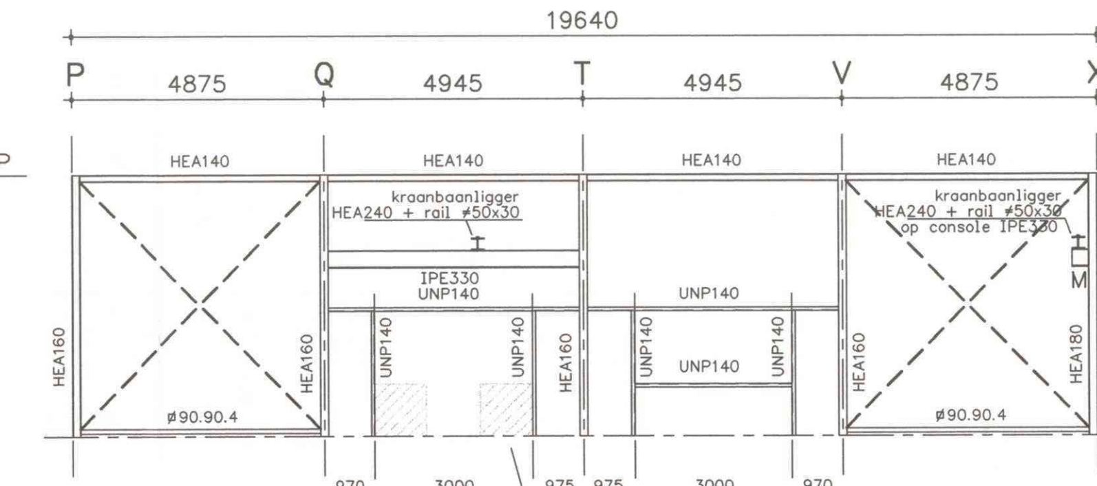
constructie in as 24: windverbanden #80x12
