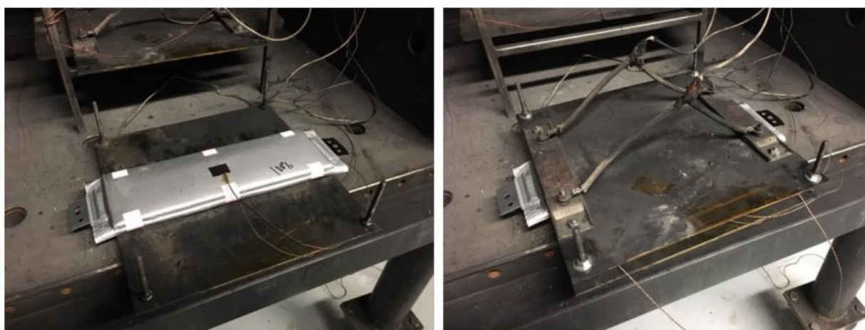
Figure 13-1: Steel plates with heaters where attached to the NMC 63 Ah pouch cells
