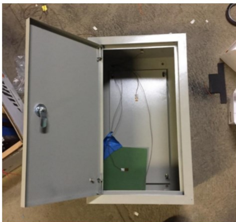
Figure 14-5 – Mild steel electrical boxes used to simulate battery module enclosures for testing.
