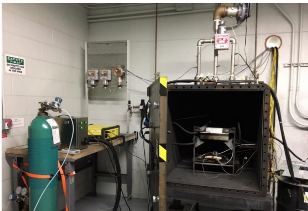
Figure 13-4 Large Destructive Test Chamber Setup
