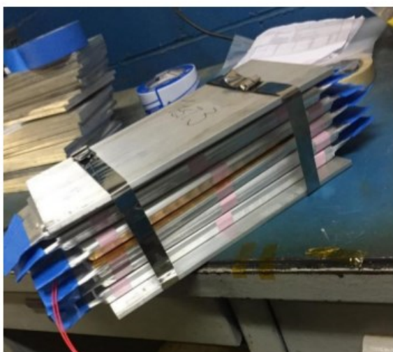
Figure 14-3 – How (NMC pouch) cells were packaged for testing – aluminum plating and stainless steel bands with resistive heaters placed in-between.
