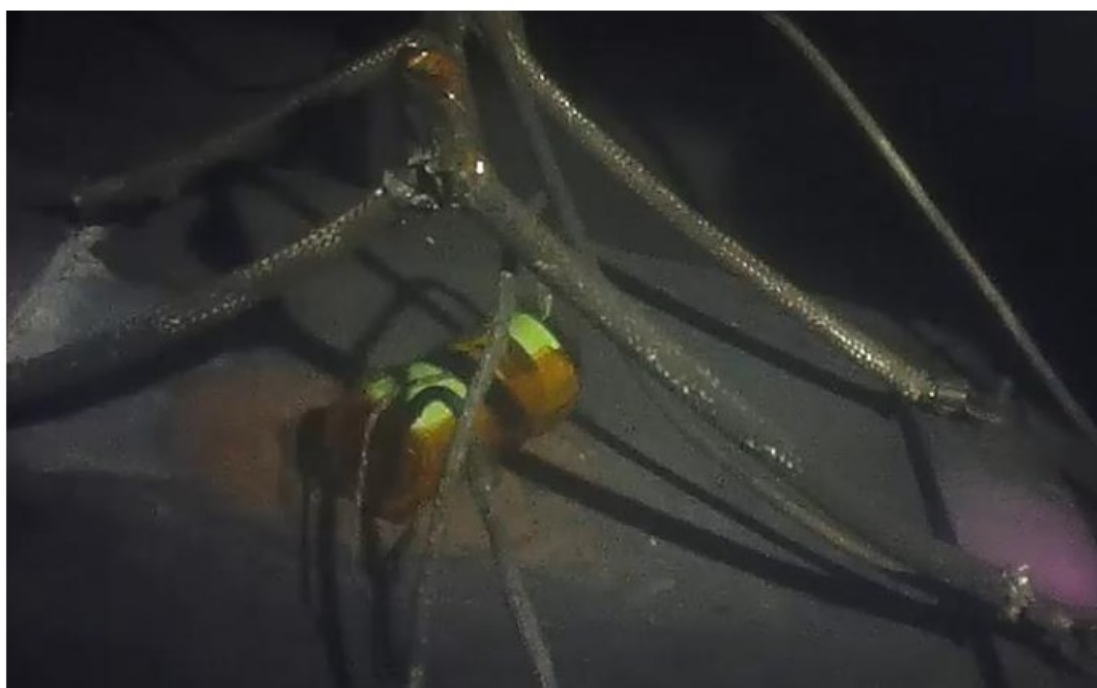
Figure 13-2: LFP 2.5 Ah cylindrical cell heated up
