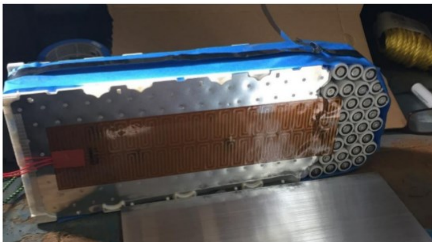
Figure 14-4 – How (LFP cylindrical) cells where packaged for testing.
