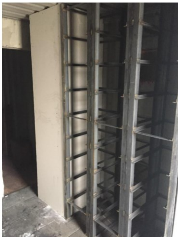
Figure 14-1 – Steel rack and drywall used to simulate battery enclosure spaces and arrangements.
