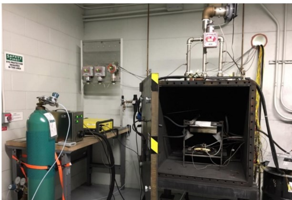
Figure 13-4 Large Destructive Test Chamber Setup
