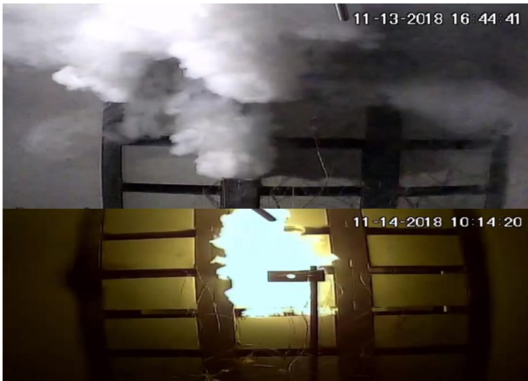
Figure 6-1 – 30 seconds after thermal runaway for a IP4X module (top) compared to a IP2X module (bottom) shows how much combustion consumes and removes gas.
