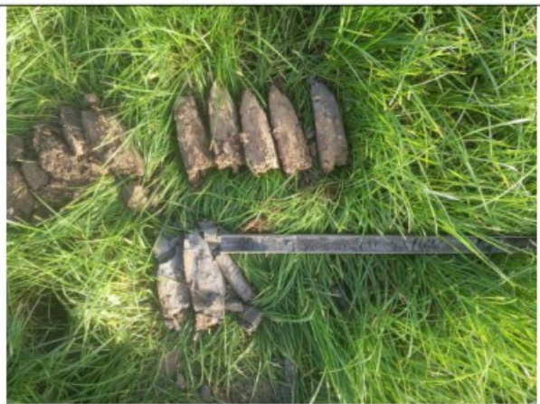
Boring 1 (bovenste 2 m, Almere Laag)
