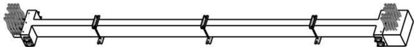
BUS BAR: 54-1016-0004 OVERALL LENGTH 4625mm SHIPPING/OPERATING WEIGHT: 598 KG
