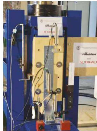
Seismic-REV experimental campaign on GL24h glulam (DICAM-University of Trento and CNR-IVALSA San 5.1.2.e Adige, 2015).
