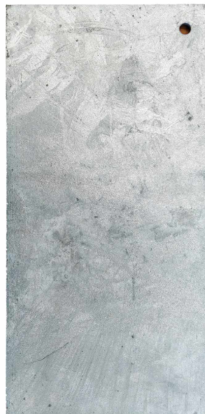
Piping, machines etc. Galvanized steel
