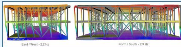
Figure 6: Natural frequencies lateral direction
